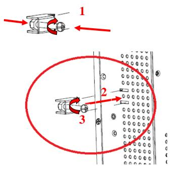
Use provided mounting kits to fix the Panel PC and the customer's fixture
